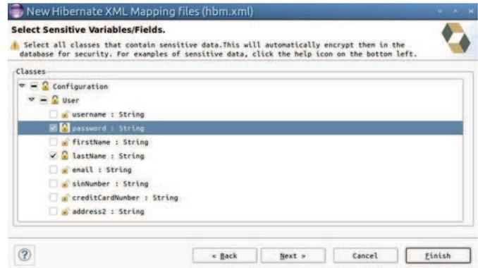
Fig. 2. Selection of fields to be encrypted.
